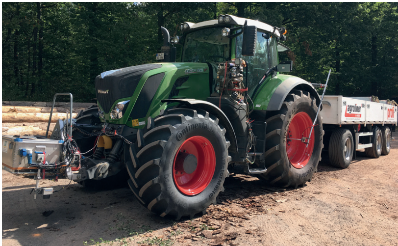
Figure 8: DLG transport test to get the fuel efficiency on the road
