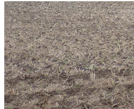
Figure 3: Soil condition at test location (wheat stubble grubbed; black earth consists of loess; middle soil humidity 10% in around 10 cm depth)
