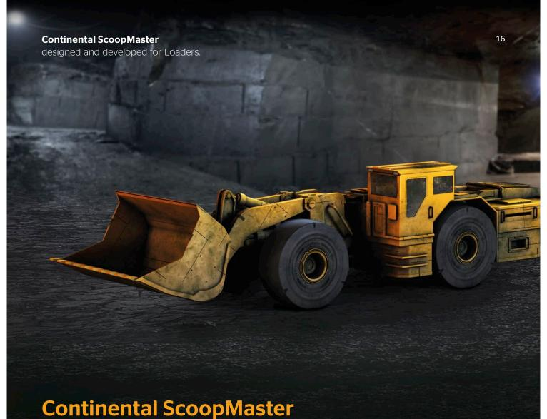
Loaders or Scoops transport heavy loads of orebodies at low speeds over a relatively short distance to dump trucks or conveyor belts. They often face freshly blasted, sharp rocks in wet and abrasive conditions. Durability, traction, and even wear are the most important tire features.
