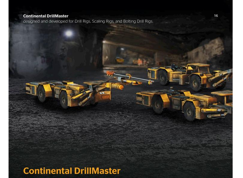
Specialized machines like Drill Rigs, Scalers, or Bolters are required for blast hole drilling in order to prepare for detonation, removal of loose rock after blasting, or the installation of rock bolts to support the roof. To drill blast holes as economically as possible, Drill Rigs cover rock cross sections of a hundred square meters and more.
