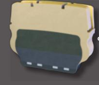
In the case of Continental's CLEAN Super Elastic Resilient tires, the tread and sidewalls are built over a multi-stage, bead wire reinforced core. The result: an extremely durable non-marking compound exterior over a shock-absorbing cushion layer and a carbon-black reinforced base.
